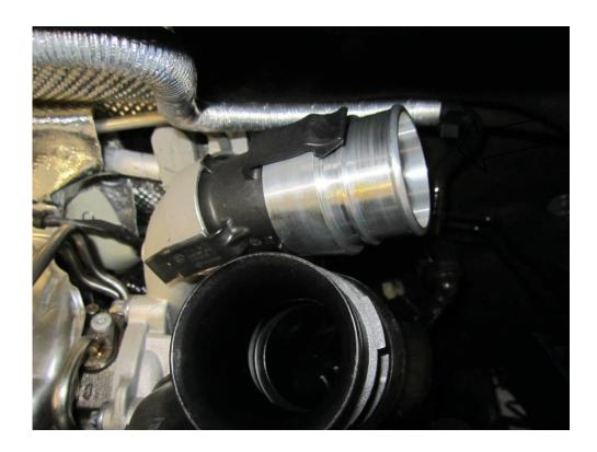
9. Now remove the OEM O-ring from the boost pipe and place it in the Forge throttle body coupler.
