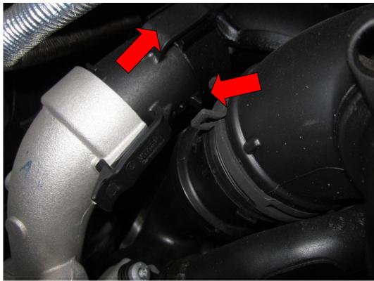
8. Insert the Forge coupler into position by pushing until you hear it click.
