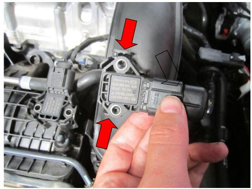
6. You can now unclip the boost pipe by prying open the tabs on the coupler joining the throttle body .
