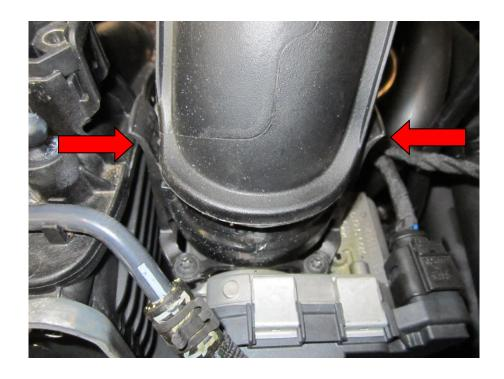
7. Unclip the opposite end of the boost pipe by again prying open the tabs arrowed red, then remove the boost pipe.
